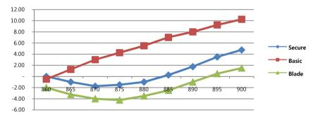
•SECURE reads up to 4.0 meters on metal, 30% longer than BASIC, but 25% shorter than BLADE. Though not best performing among similar size tags, its performance is most stable and consistent, as its slow and gentle slope of sensitivity curve shows.
