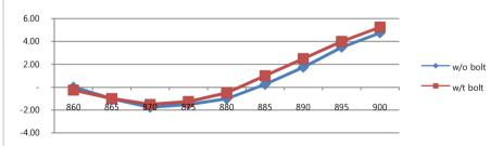
•SECURE reads same, regardless of whether it is fastened with metal bolt in two holes (located on center of both ends) or not. Stainless steel M3 bolt with round head is best fit for SECURE.
